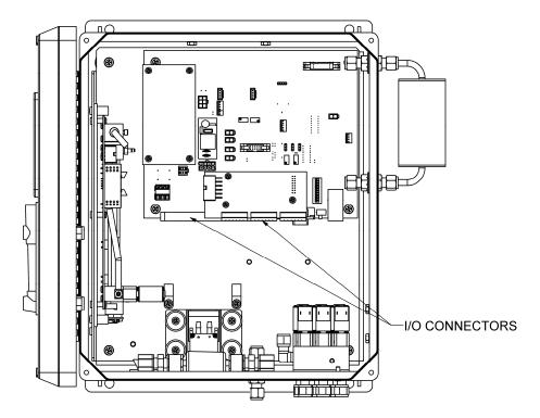
Figure 4-7: NEMA Electrical I/O Connections
